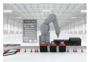
**Photo 1:** The innovative Linear Transfer System offers greater production line flexibility by using on-board intelligence and connectivity to allow each Smart Carriage to behave differently and autonomously. [Source: Mitsubishi Electric Europe B.V., Getty Images]
